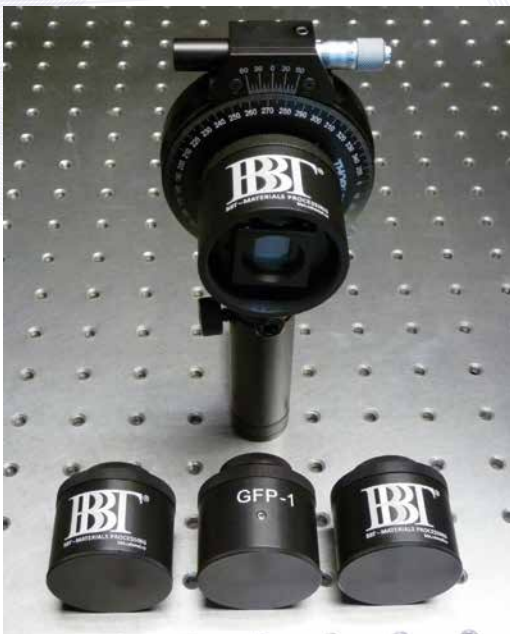
Calomel based Glan-Foucault polarizer for infrared region.
